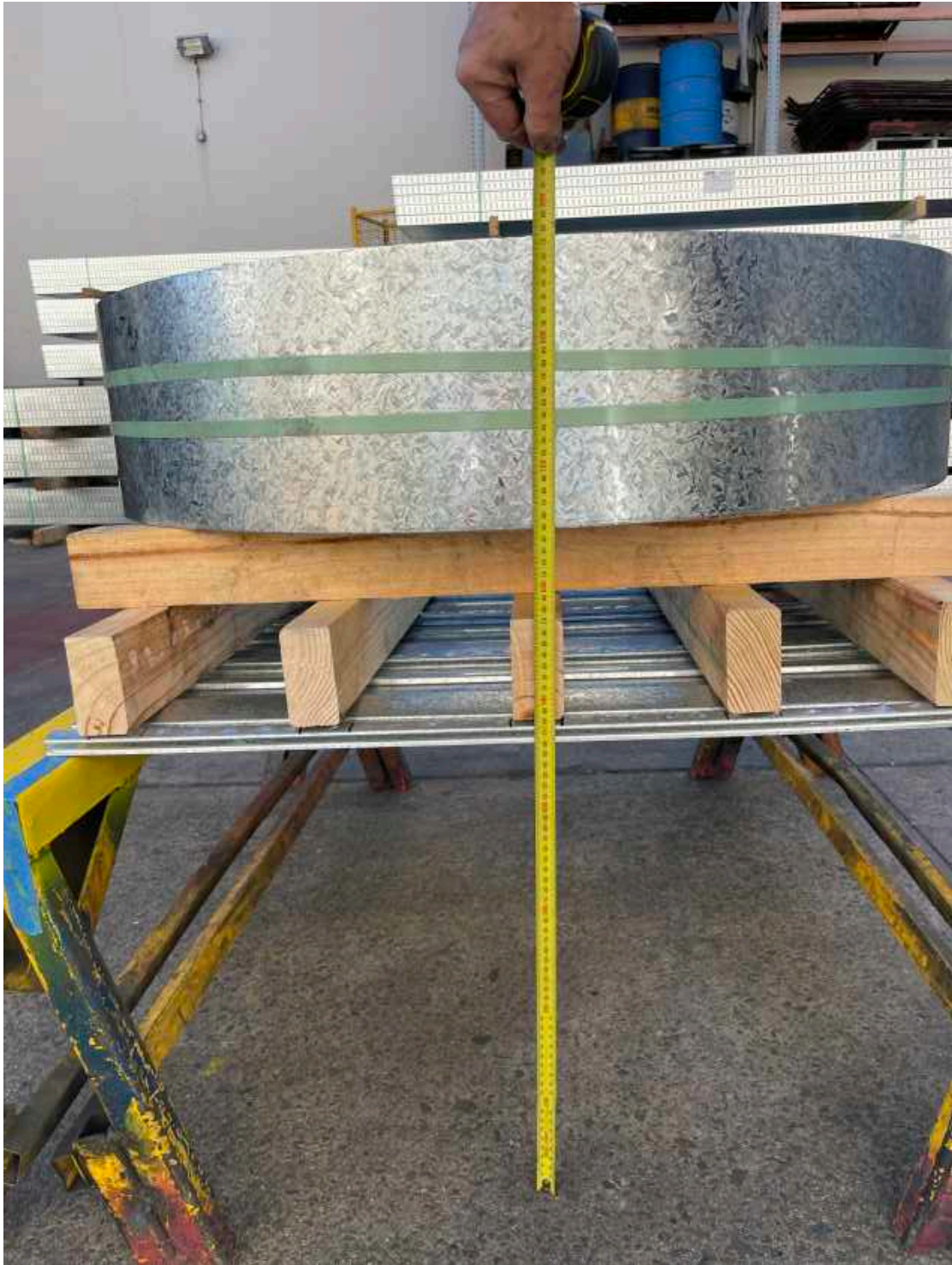
Photo 3: The deflection on the 0.75mm BMT PremierDek 20 at time of loading.
