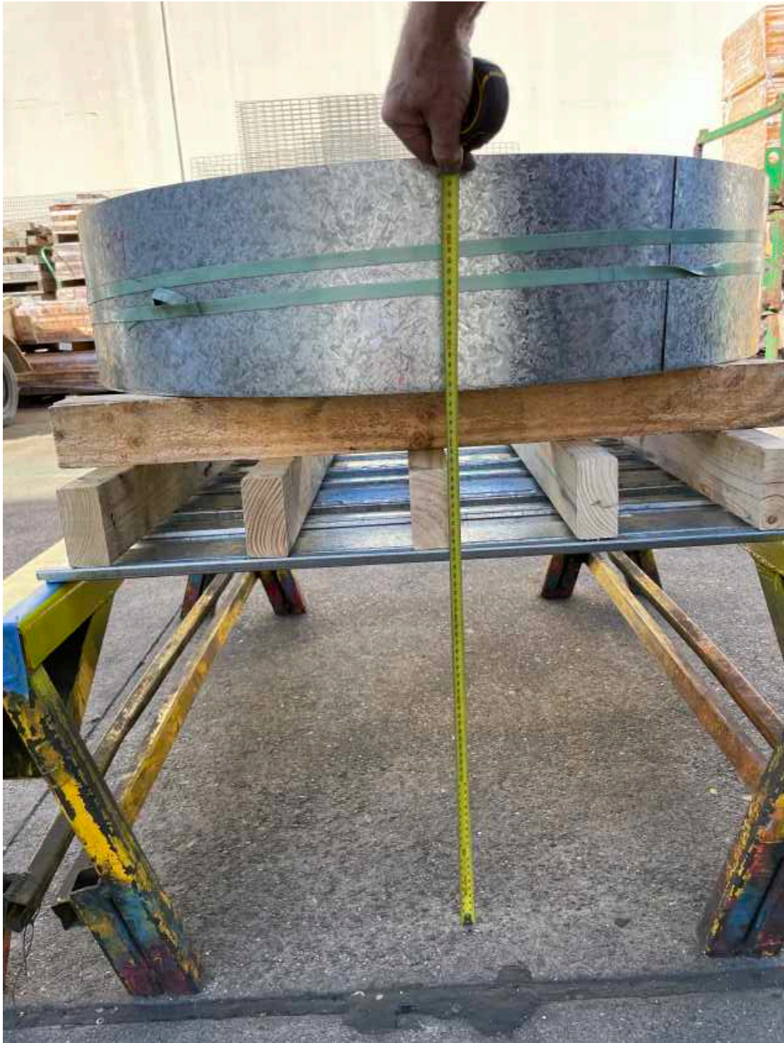
Photo 5: The deflection on the 0.75mm BMT PremierDek 20 at time of loading.
