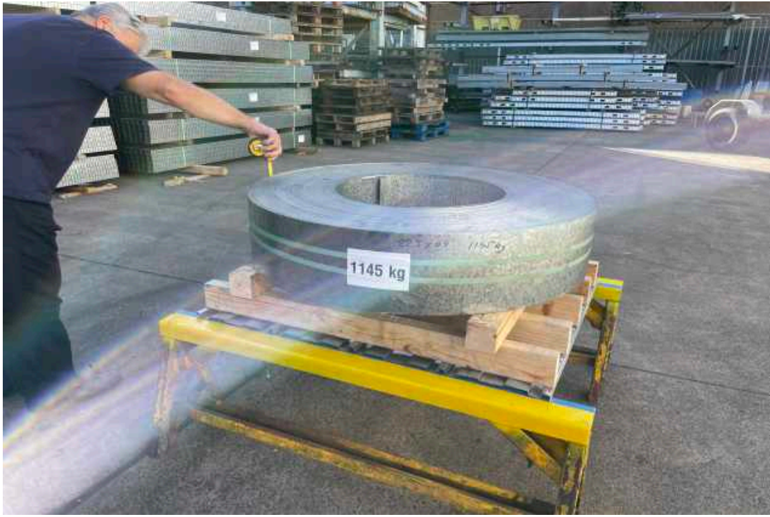
Photo 2: The steel 1145kg steel coil and timber loading.
